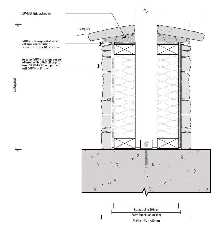
Note: THIS DETAIL DOES NOT HAVE CAVITY BATTENS
